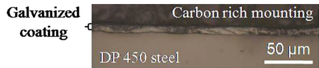
Fig. 5—Transverse cross section of the galvanized DP450 steel (light microscopy).
