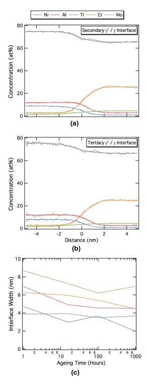
Fig. 7— Proximity histogram of elemental concentrations across the secondary  $\gamma'/\gamma$  interface (a) and the tertiary  $\gamma'/\gamma$  interface (b) for the alloy aged for 16 h. (c) The variation of the secondary  $\gamma'/\gamma$  interface width as a function of aging time (Color figure online).
