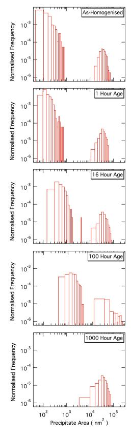
Fig. 2— Particle size distributions (PSDs) of the  $\gamma'$  precipitates in the as-homogenized state and after aging for 1, 16, 100, and 1000 h at 1033 K (760 °C) (Color figure online).
