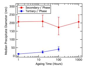
Fig. 3— Mean diameters of the secondary and tertiary  $\gamma'$  precipitates as a function of aging time at 1033 K (760 °C) (Color figure online).
