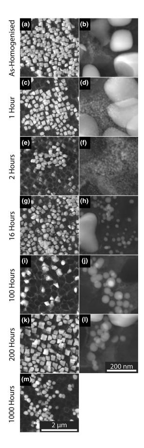
▼ Fig. 1— STEM images of extraction replicas of alloy in the as-homogenized state (a, b) and after 1 (c, d), 2 (e, f), 16 (g, h), 100 (i, j), 200 (k, l), and 1000 (m) h of aging at 1033 K (760 °C). Secondary γ′ precipitates are shown on the left-hand side (a, c, e, g, i, k, m) and tertiary γ′ precipitates on the right-hand side (b, d, f, h, j, l). No tertiary precipitates were visible after 1000 h of aging.
