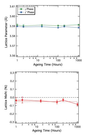
Fig. 8— Variation of the lattice parameter of each phase, and the lattice misfit of the alloy as a function of aging time at 1033 K (760 °C). The average lattice misfit during aging is shown as a dotted line (Color figure online).
