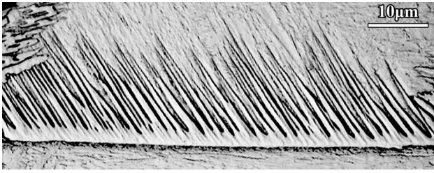
Fig. 28—Semifeather, a wide group of parallel plates on one side of a grain boundary and formed from individual nuclei, which have later merged to a seeming grain boundary film. From 923 K (650 °C) after 2 s.
