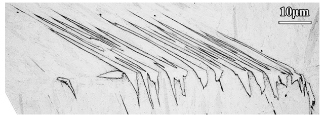
Fig. 26—Wide group of parallel plates formed from grain boundary after 2 s at 973 K (700 °C). The nuclei have developed as sawteeth in the other grain, probably with their main growth direction at a large angle to the plane of polish.
