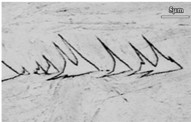
Fig. 23—Sawteeth after 1.5 s at 973 K (700 °C) starting to merge. Plate-like outgrowths formed mainly before the quench.
