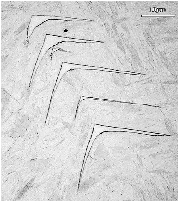
Fig. 20—Chevrons formed after 1.5 s at 973 K (700 °C). The inner corners are in the process of being filled.
