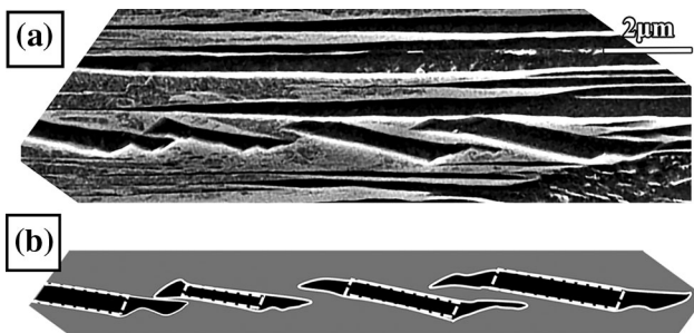
Fig. 43—(a) Cross sections of four plates from 773 K (500 °C). (b) Suggested initial cross sections and protrusions.
