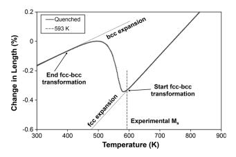
Fig. 2—Change in length vs temperature during cooling at 20 K s<sup>-1</sup>.
