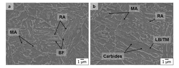
Fig. 7—Different microstructures obtained in a specimen isothermally treated just at  $M_s$  at 593 K (320 °C) for 3600 s. Bainitic Ferrite is indicated by BF, Martensite-Austenite islands by MA, Retained Austenite by RA, and Lower Bainite or Tempered Martensite by LB/TM.
