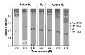
Fig. 10—Phase fractions obtained after the application of selected heat treatments including isothermal treatments at temperatures above, just, and below  $M_s$ . Prior athermal Martensite is indicated by PM, Bainitic Ferrite by BF, Fresh Martensite by FM, and Retained Austenite by RA.
