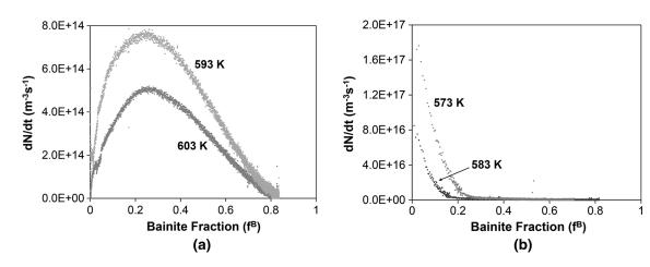
Fig. 13—Evolution of nucleation rates during different isothermal holdings at temperatures above and just at  $M_s$  (a) and below (b) the  $M_s$  temperature, assuming a temperature-dependent volume of the bainitic subunits.
