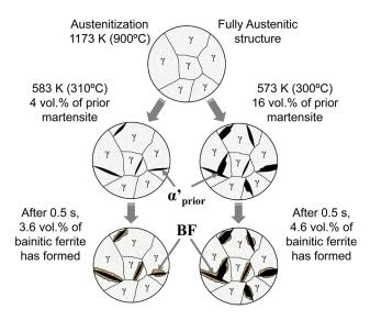
Fig. 15—Schematic evolution of the initial microstructure at the very beginning of the isothermal holding at temperatures 583 K and 573 K (310  $^{\circ}$ C and 300  $^{\circ}$ C), both below  $M_{s}$ .
