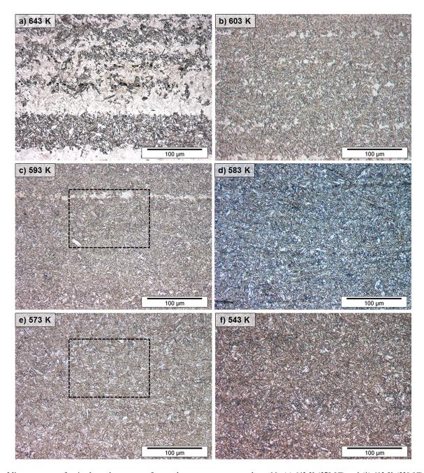
Fig. 4—Microstructures after isothermal treatments for one hour at temperatures above  $M_s$ , (a) 643 K (370 °C) and (b) 603 K (330 °C), just at  $M_s$ , (c) 593 K (320 °C), and below  $M_s$ , (d) 583 K (310 °C), (e) 573 K (300 °C), and (f) 603 K (330 °C). The dashed rectangles are enlarged in Figs. 5(a) and (b), respectively.
