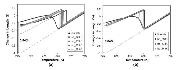
Fig. 9—Change in length as a function of temperature for isothermal treatments above and just at  $M_s$  (a) at 643 K, 613 K, 603 K, and 593 K, (370 °C, 340 °C, 330 °C, and 320 °C) and below  $M_s$  (b) at 583 K, 573 K, and 543 K (310 °C, 300 °C, and 270 °C).
