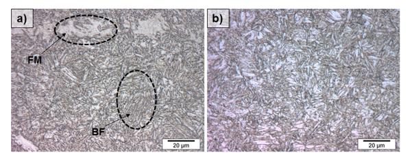
Fig. 5—Enlarged images of the area surrounded by dashed squares in Figs. 4(c) and (e), corresponding to the microstructures obtained in specimens isothermally treated for 3600 s: (a) just at  $M_s$  at 593 K (320 °C), and (b) below  $M_s$  at 573 K (300 °C). Bainitic Ferrite is indicated by BF, and Fresh Martensite by FM.
