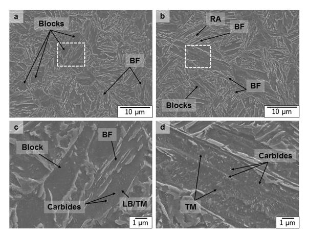
Fig. 8—(a) and (b) Microstructures obtained in a specimen isothermally treated below  $M_s$  at 573 K (300 °C) for 3600 s. (c) and (d) Enlarged images of the area surrounded by a dashed square in (a) and (c), respectively. Bainitic Ferrite is indicated by BF, Retained Austenite by RA, Lower Bainite or Tempered Martensite by LB/TM, and Tempered Martensite by TM.
