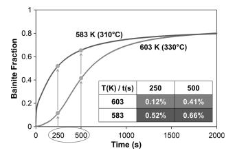
Fig. 12—Bainite fractions as a function of time at 603 K and 583 K (330 °C and 310 °C), above and below the  $M_{\rm s}$  temperature, respectively.
