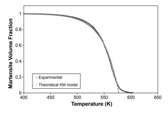
Fig. 3—Experimental volume fraction of martensite calculated applying the lever rule and fitting of this volume fraction by the Koistinen and Marburger model.
