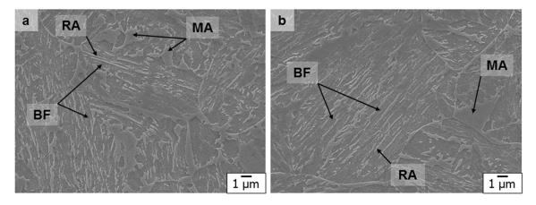
Fig. 6—Microstructures obtained in a specimen isothermally treated above  $M_s$  at 613 K (340 °C) for 3600 s. Bainitic Ferrite is indicated by BF, Martensite-Austenite islands by MA, and Retained Austenite by RA.
