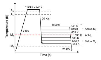
Fig. 1—Schematic representation of heat treatments applied to the selected steel.
