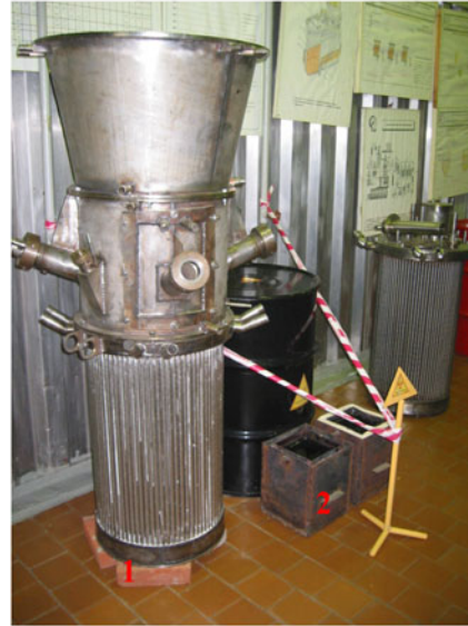
Fig. 5—(a) JHCM melter at Nuclear Research Centre (FZK), Karlsruhe, Germany for vitrification of highly active waste concentrate (HAWC). [48] Courtesy S. Weisenburger, Forschungszentrum Karlsruhe. (b) A view of a CCM (1) and rectangular carbon steel containers (2) used at Moscow SIA “Radon” for vitrification of LILW. [13]
