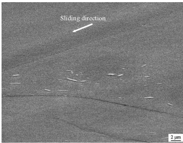
Fig. 6—SEM micrograph of the wear track on the surface of the Ti-Mo-N film at f_{N_2} = 2.0 ccm.
