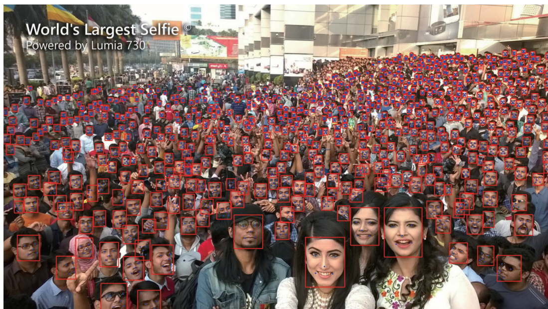
Fig. 6 The world's largest selfie. Our YuNet successfully detects 619 faces out of approximately 1 000 faces reported. The undetected face contains only a few pixels, is blurred and can not be recognized by human eyes. They can be directly ignored in real applications.
