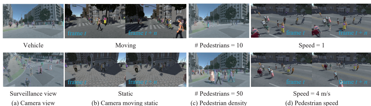
Fig. 2 MOTX is inexpensive and accurate in generating videos and their labels for association training. Controllable factors include (a) camera view, (b) camera moving state, (c) pedestrian density, and (d) pedestrian speed.
