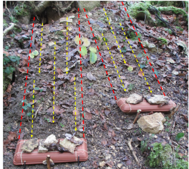
Fig. 3 Sediment traps were positioned at the base of fresh soil mounds on the down-valley side and kept in place using wooden pegs and stone weights. Upslope runoff generation areas are depicted in red dashed lines, and possible flow-paths depicted in yellow dashed arrows.
