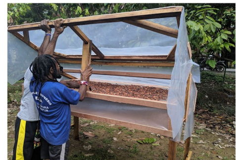
(b) Implemented solar dryer solution for cocoa farmers in Mimika.
