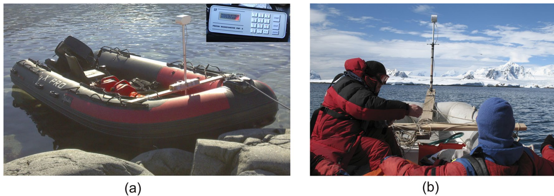
Fig. 4 Boat Zodiac with set up of proton magnetometer PMP-8 used for the magnetic survey. Shows the mounting of the magnetometer sensor on the Zodiac rubber boat, and a panel of PMP-8 (top right
