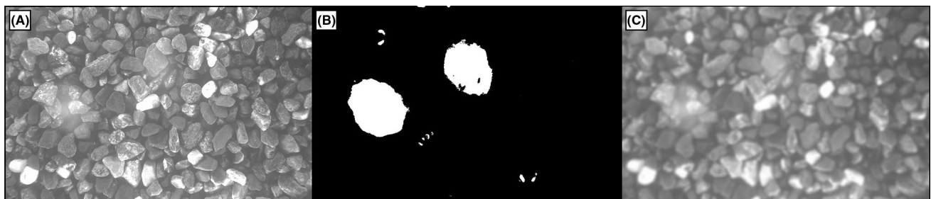
Fig. 3 A Original image from the video. B Binary version of the image with two false detected particles. C Blurred, 2D Gaussian filtered version of the original image to decrease noise without losing information in the LSPIV and SBM
