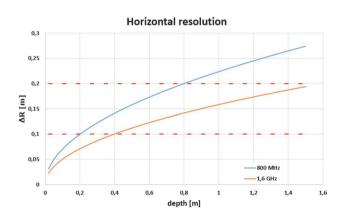
Fig.4 Dependency of the horizontal resolution on the depth for antennas of different frequencies
