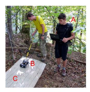
Fig. 5 Field measurements setup. a ProEx System in the backpack; b HF antenna, c PCV measuring mat (photograph by J. Karczewski)
