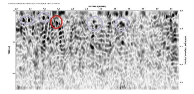
Fig. 8 Radargram of the profile 7 in the FIELD1 with purple circles indicating weathered melaphyres and tree roots and red circle indicating an agate
