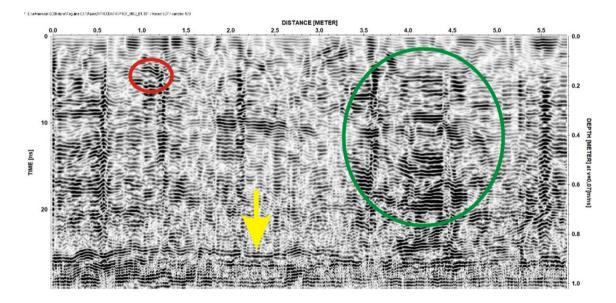
Fig. 10 Radargram of the profile 2 in the FIELD2 with green ellipse indicating tree roots and red ellipse indicating a multicolored agate
