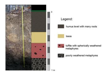
Fig. 3 The geological column of a point at the measurement site
