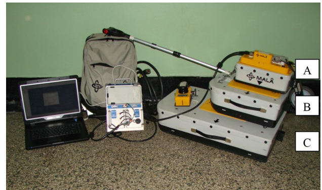
Fig. 3 GPR system (ProEx system) with different antennae (800 MHz— a ; 500 MHz— b and 250 MHz— c )
