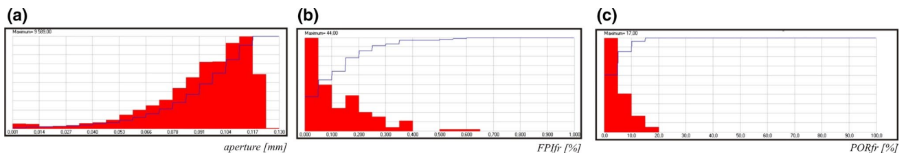
Fig. 8 Histograms of: a fracture aperture; b FPI values; c fracture porosity laboratory data
