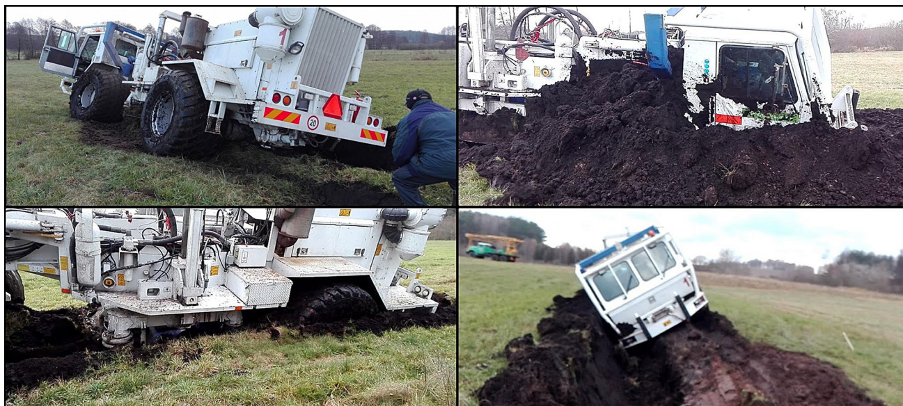
Fig. 1 Examples of field condition during acquisition. From the beginning of October, up to the time of acquisition (November), as well as during them, there were significant rainfalls, which resulted in very difficult terrain conditions. The ground was soaked with water. This caused the vibroseis to sink into the soaked ground dur-
