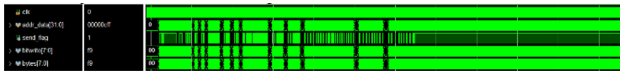
Fig. 20 Entropy encoding results comparison diagram, Can see that the value of the codestream output by the JPEG XS entropy encoding top module is the same as the value of the codestream output by the reference software
