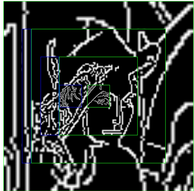
Fig. 24 Canny feature extraction at multiresolution levels of the MMMF approach with sending blocks
