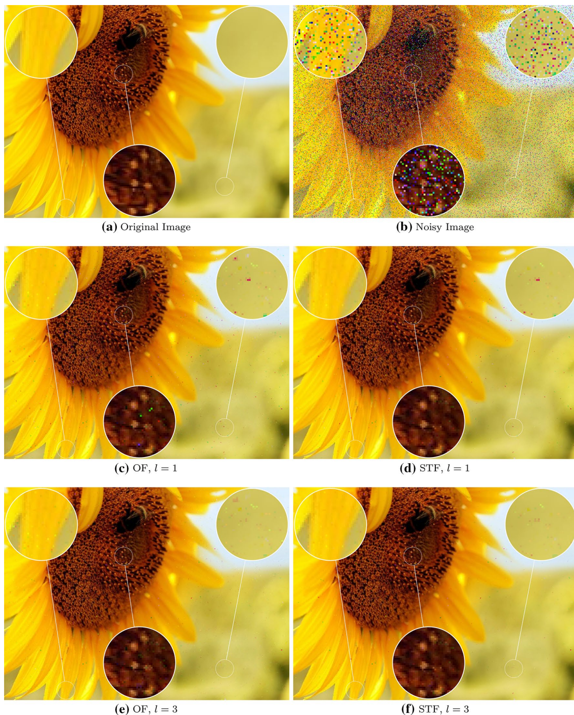
Fig. 12 Visual comparison of OF and STF performance for \rho = 30\% and validation image 8
