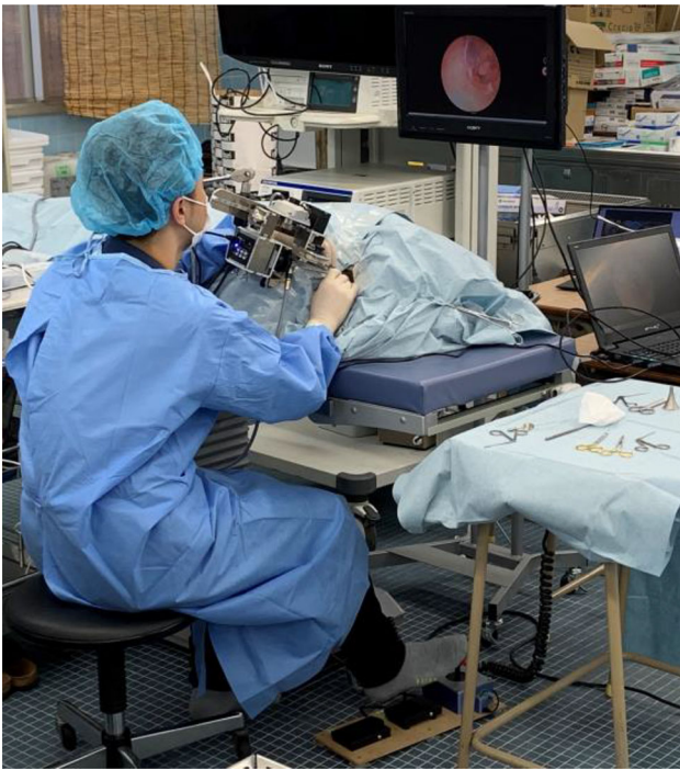
Fig. 1 Simulated surgery performed by an otologic surgeon using an endoscope manipulator for TEES with gimbals rotation and linear rail mechanism driven by DC servo and ultrasonic motors
