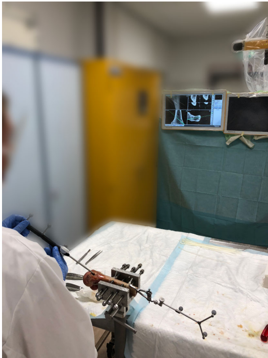
Fig. 2 The experimental setup during navigated curettage of a distal femur. The surgeon uses the tracked pointer to assess the tumor shape and location
