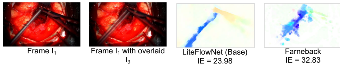
Fig. 1 Test sequence in our evaluation data with corresponding plots for two calculated optical flow, LiteFlowNet and Farneback, and interpolation error (IE). Optical flow is converted to polar space for visualization using HSV space, whereas hue encodes pixel-wise vector direction and saturation is used to show pixel-wise vector magnitude
