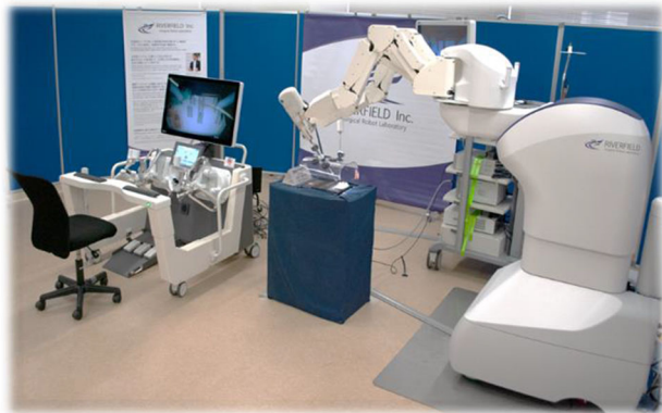
Fig. 1 Surgical robot with grasping force feedback named Saroa
