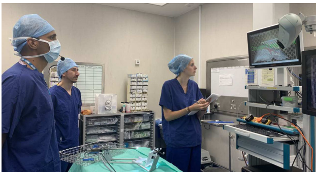
Fig. 3 The SmartLiver system being tested in theatre with a voice-controlled user interface. The SciKit-Surgery architecture allows the SmartLiver system to be easily connected to the scikit-surgeryspeech library, to test the effectiveness of voice control for calibration and manual alignment
