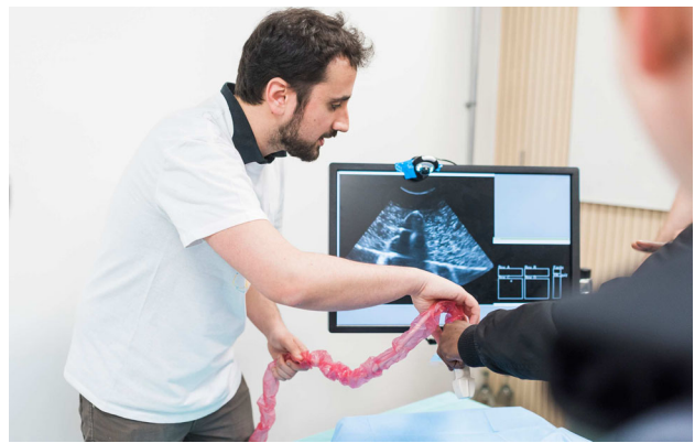
Fig. 4 SnappySonic in use at the Science of Surgery public engagement event. An obsolete ultrasound probe is tracked using OpenCV's ArUco marker libraries. The position of the probe is used to show an image from a pre-recorded ultrasound buffer, giving the appearance of live acquisition. Image by James Tye
