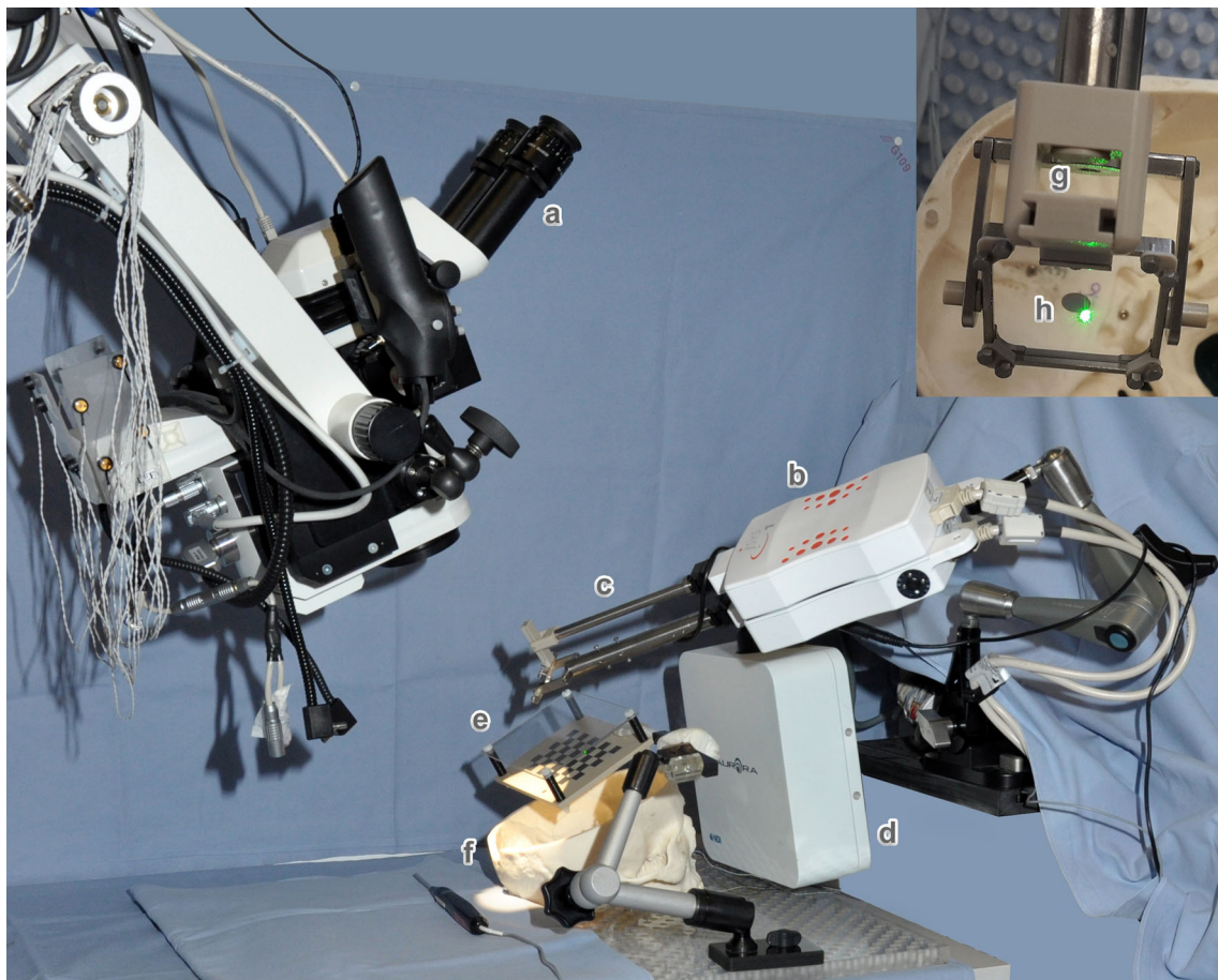
Fig. 1 Components of the prototype setup: a Leica M500N stereo microscope with HD cameras, b iSYS-1 robot platform, c custom-built end-effector (medical grade-1 titanium and PEEK) housing a green laser in the lower shaft, d NDI Aurora field generator, e acrylic glass/PEEK dual plate for laser tracker co-alignment, f plastic skull with implanted
