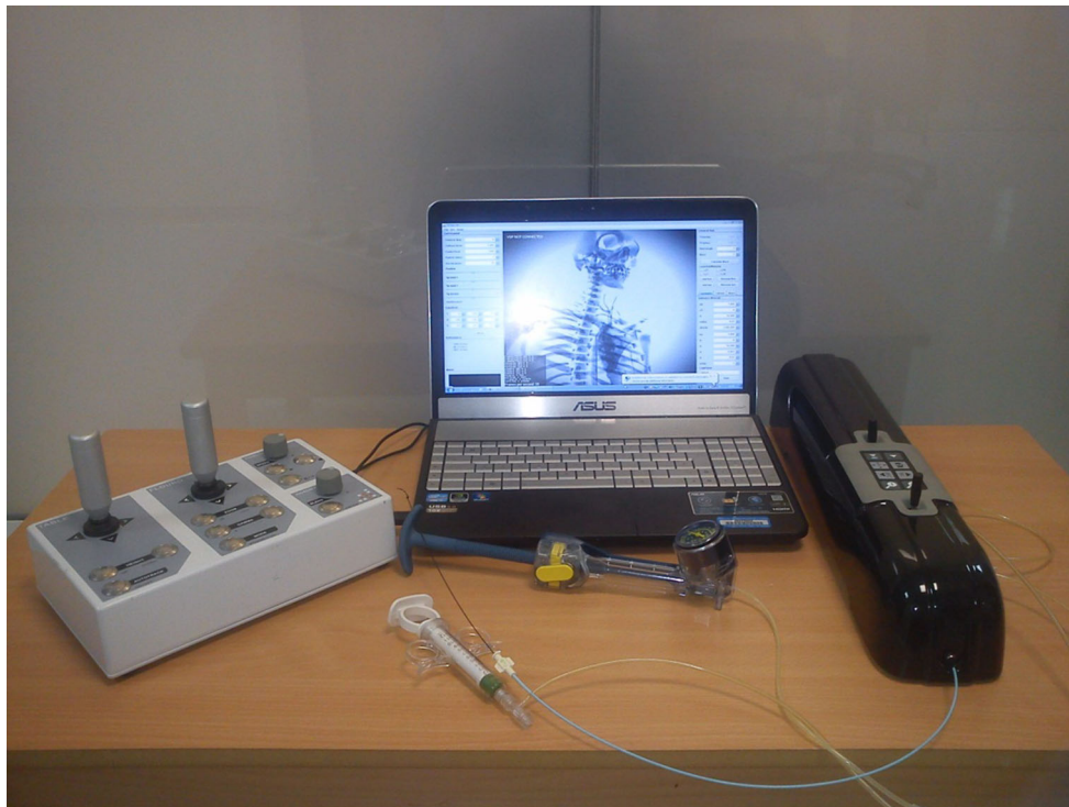
Fig. 1 VCSim3 complete set-up including the simulator software running on the laptop, VSP haptic device, fluoroscopic view console, balloon inflation device, and contrast injection syringe
