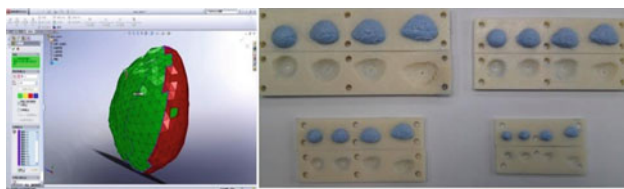
Fig. 2 Design and rapid prototyping the mold for 3D tumor phantom with various shapes and sizes
