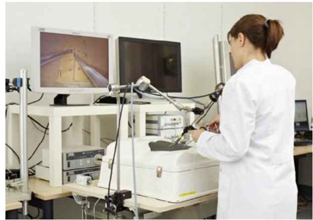
Fig. 2 Experimental setup for evaluation of different 3D and a 2D laparoscopic monitors. Subjects had to complete a laparoscopic suturing task under standardized conditions. Procedure time, electromagnetic tracking of instruments and accuracy of suturation were assessed as performance parameters, while the NASA TLx score provided information concerning the mental work load. To prevent bias laparoscopic cameras and video devices were identical among the different workplaces (Karl Storz® 3D TIPCAM NTSC)
