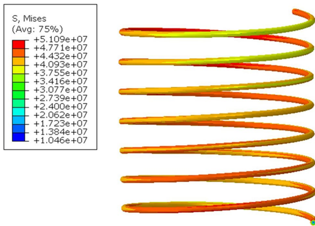
Fig. 8 Spring stress results at max operating conditions of 2.22 mm displacement
