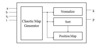
Fig. 1 Generation of key and position map using chaotic map
