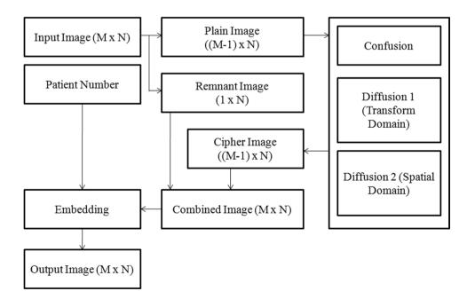
of the DICOM image after decryption. This is because the first row is excluded during the encryption process. The
