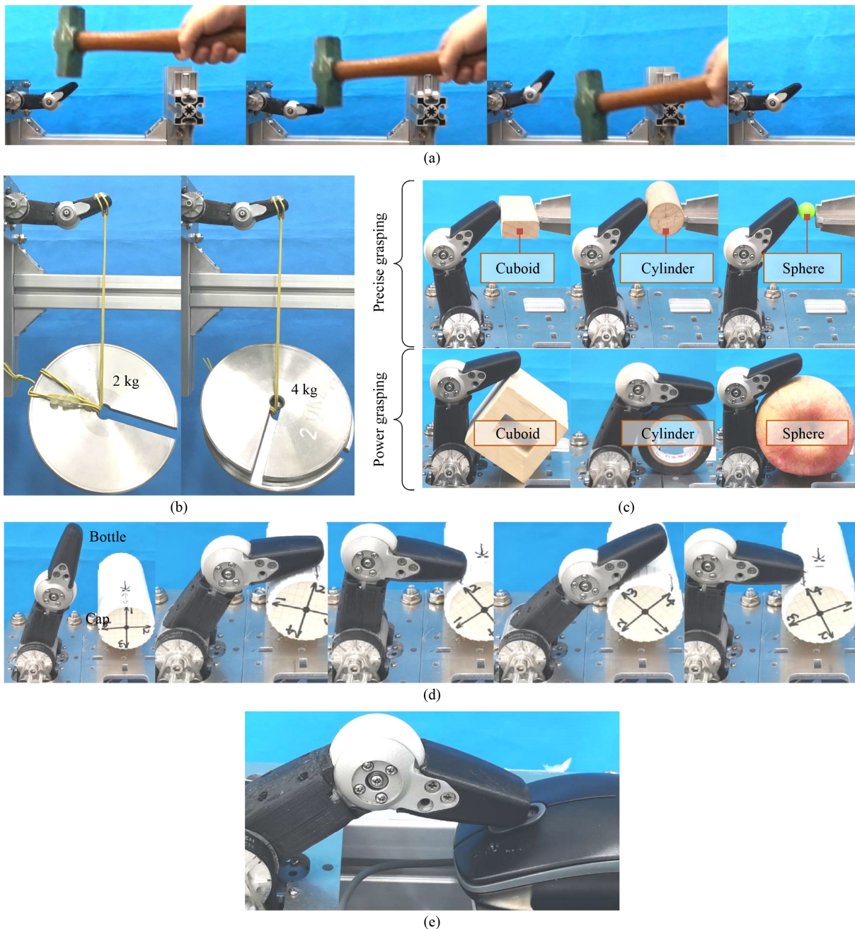
Fig. 15 Physical impact, lifting, grasping, and manipulating tests. (a) Hammering the finger with a steel hammer at a speed of 1.2 m/s, (b) lifting tests, (c) precise grasping and power grasping, (d) screwing the cap, and (e) clicking the roller of the mouse.
