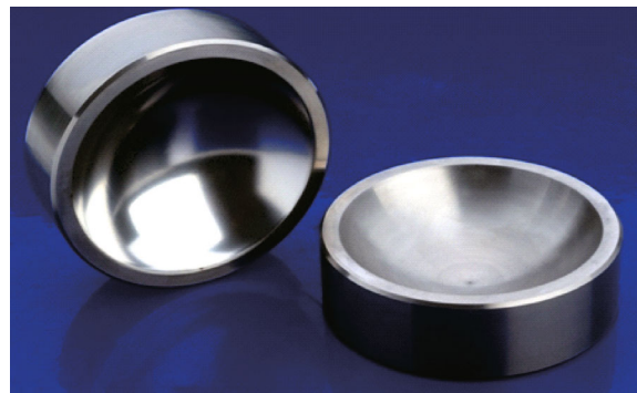
Fig. 18 Laser polished spherical cap (on left) and initial surface (right) [94]
