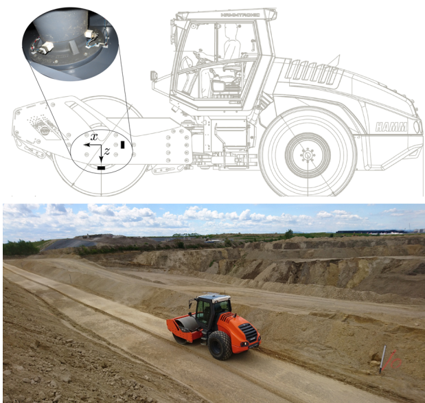
Fig. 1 Measurement setup and definition of directions x and z in the experimental field tests (top), and photograph of the experimental field test (bottom)
