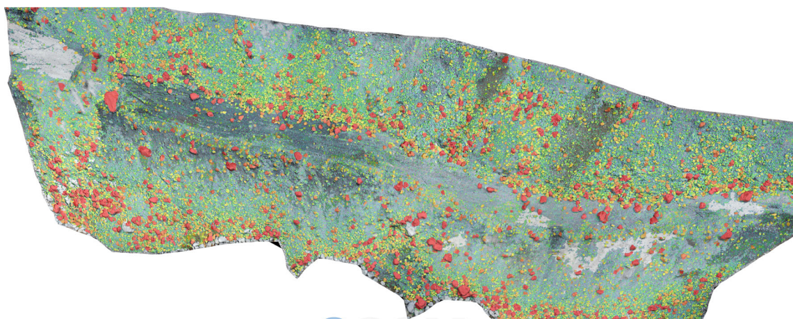
Fig. 8 Detailed 3D model of waste dump WD-5, featuring over 7 million points and 2.6 million mesh elements
