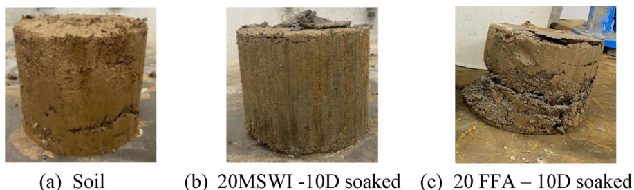
Fig. 11 Samples after 10 days soaking a soil b 20MSWI fly ash and c 20FFA
