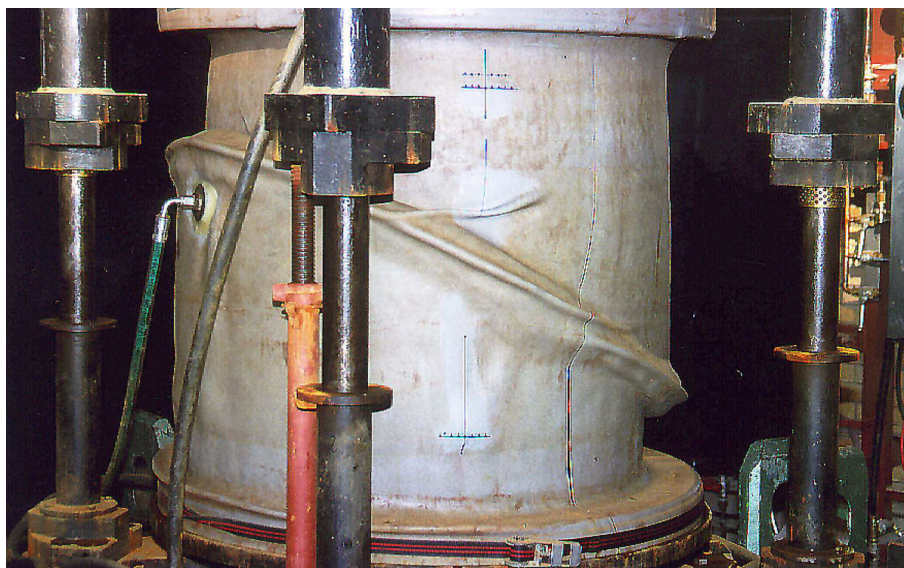
Fig. 6 Sample of gravel with an embedded inclined clay disc, taken from an open-cast mine and re-compressed after remoulding, enclosed by a membrane with 80 cm diameter, after axial loading via smooth end plates with central drainage holes, with confining pressure and hydraulic gradients as under the open-cast mine referred to in Sect. 5
