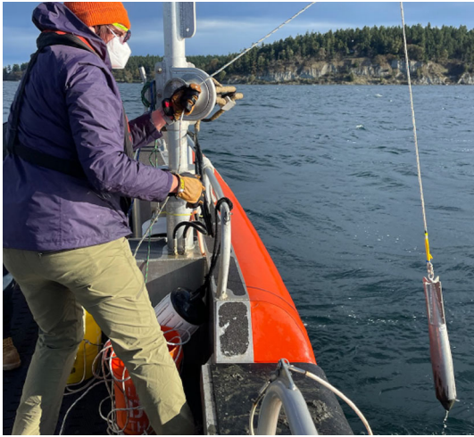
Fig. 2 The portable free fall penetrometer BlueDrop during deployment
