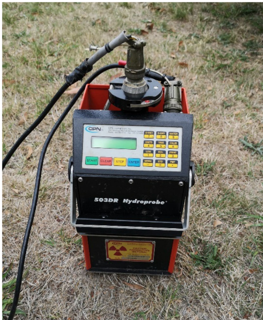
Fig. 5 Neutron moisture meter (Campbell Model 503DR) used to determine soil moisture levels in the vicinity of a C. maculata tree
