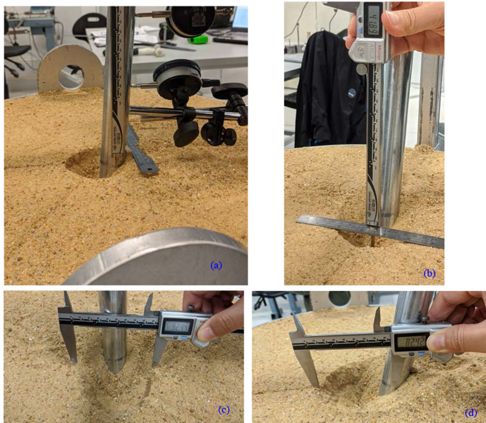
Fig. 7 Soil displacement at the ground surface around the pile in test RP3 at 165.6 N
