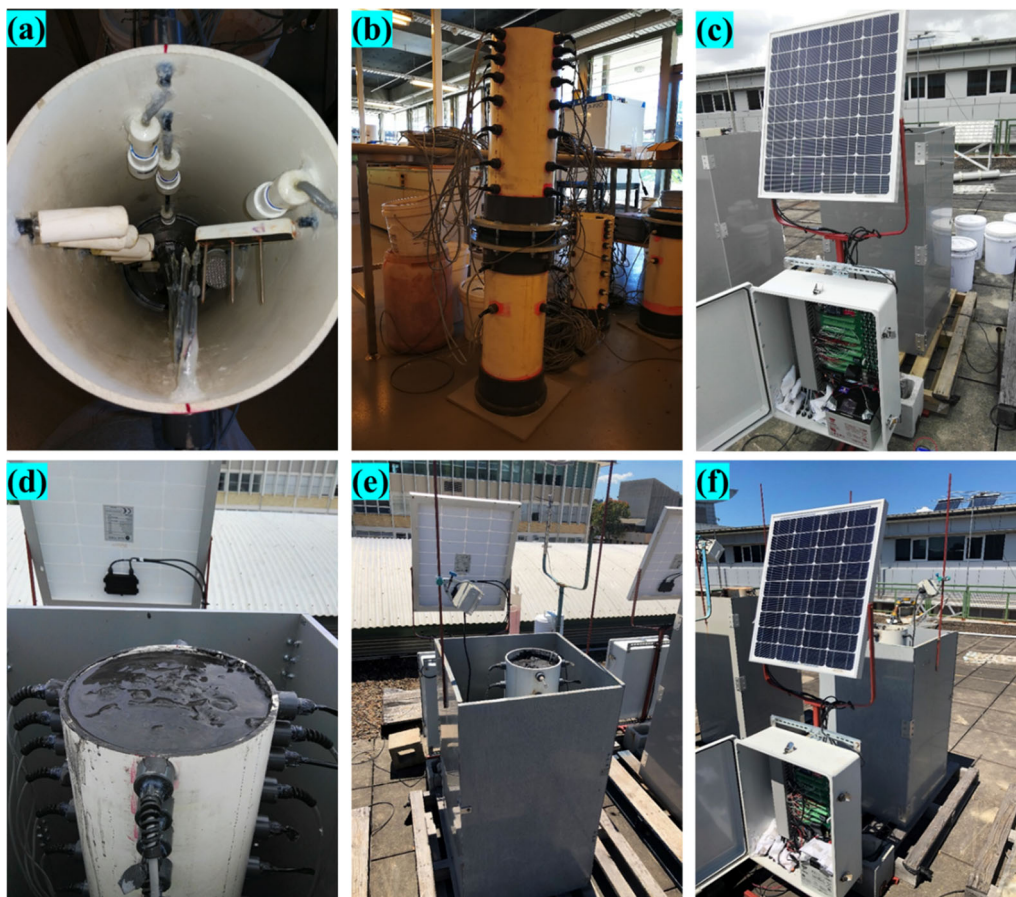
Fig. 4 Images of the instrumented column assembly processes: a top view of sensors layout before deposition of tailings; b assembled column with sensors installed; c rear view of the column (enclosed by four PVC panels), solar panel and electrical enclosure; d top view of the column after the additional top section being removed; e front view of the column after the top 150 mm section being trimmed in March 2019; f rear view of the trimmed column
