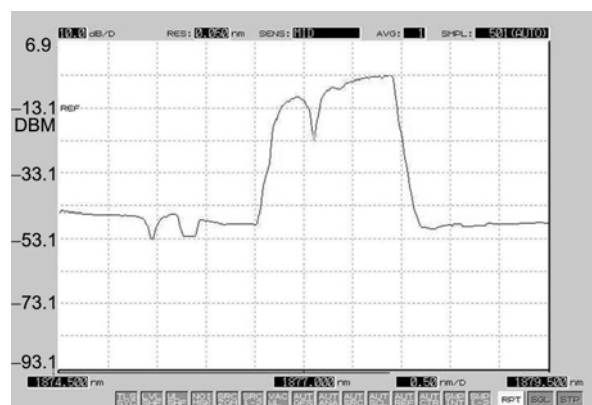
Figure 7 1877 nm absorption spectrum with the “maxhold” function selected.
