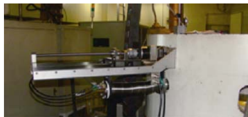
Figure 9 Structure of the radial probe.
