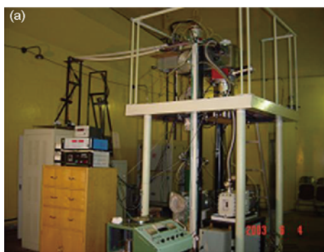
Figure 1 A picture of the test stand for H^- ion source (a) and a cross section of the extracted beam (b).
