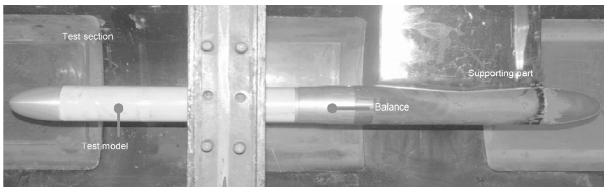
Figure 10 Test model and its installation.
