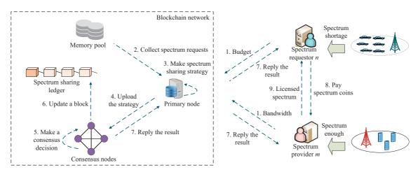
Figure 6 (Color online) Blockchain-enabled DSS workflow.
