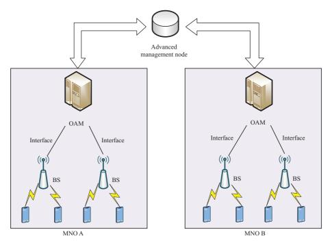
Figure 2 (Color online) Centralized DSS architecture.
