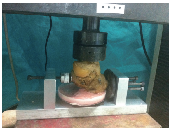
Figure 6 (Color online) In vitro experiment using a material testing machine on a calcaneal specimen.
