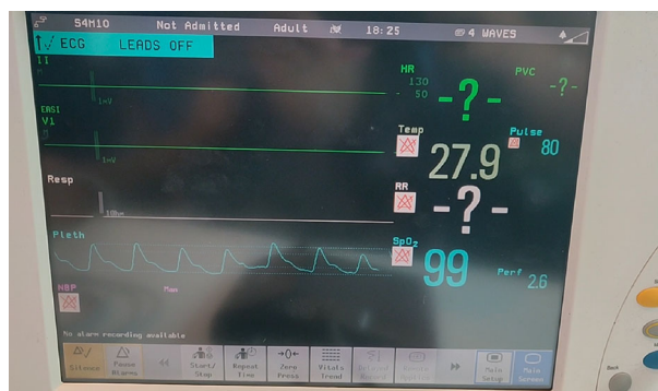
Fig. 15 Patient vitals and other information shown on the display of the Philips MP50 patient monitor. The pulse rate reading (80 beats per minute) is displayed on the right-hand side of the screen. The pulse is measured by the finger plethysmograph that is attached to one of our fingers, simulating an actual patient being monitored. Some vitals are missing (value set to -?-) because the sensors are not connected to the patient monitor
