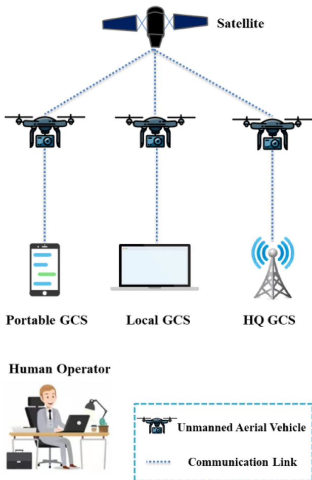
Fig. 3 Architecture of UAV system
