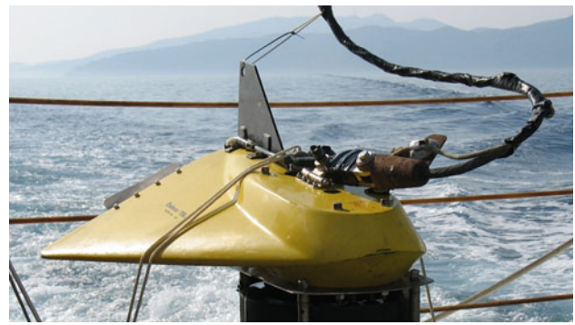
Fig. 4 Our echo repeater, used to simulate an underwater target
