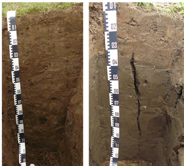
Fig. 9 Soil profile view of test cell 1 (left, marsh sediment) and test cell 2 (right, marsh sediment + dredged material), excavated in 2012, eight years after construction
