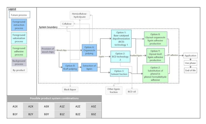
**Fig. 4** Flow chart showing all considered production pathways for lignin. The possible future combinations of the production processes are in the lower left corner of the figure. Processes that are highlighted with dark
