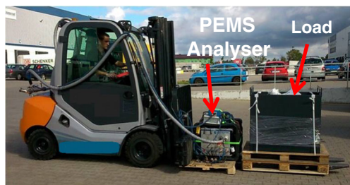
Fig. 1 The installation of the measuring equipment on a forklift truck
