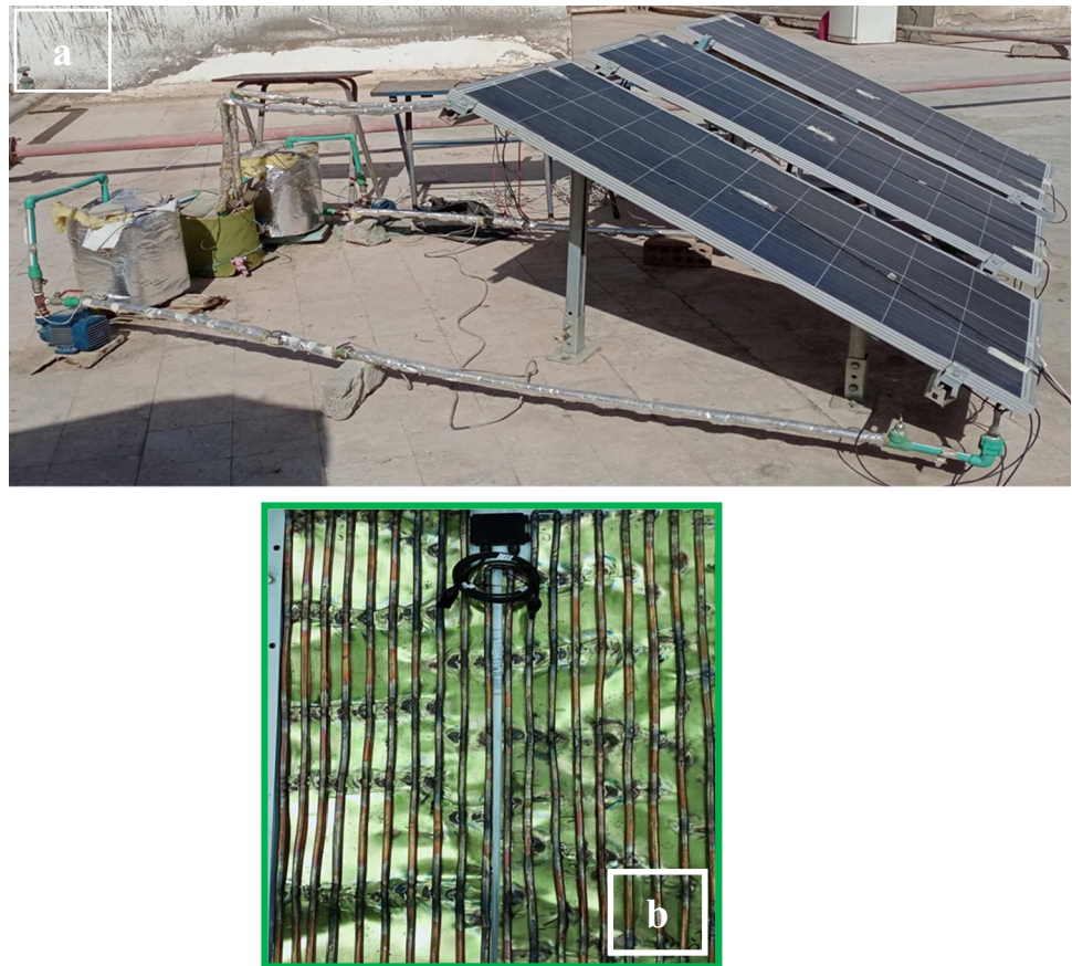
Fig. 2 Photograph of assembly of various components of a PVT system. (a) Whole PVT system. (b) Serpentine heat exchanger at the back of the solar panel
